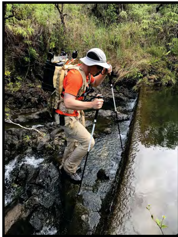
Figure 3: Brett Connell using Backpack HDSS on Paakea Stream, Maui. The GPS-linked video cameras are image stabilized to dampen the bounces associated with walking in a stream.
